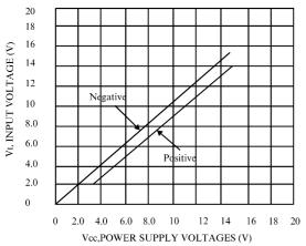
Figure 1.Input Voltage Range
