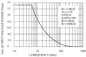
Figure 3. Large-Signal Frequency Response
