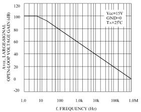
Figure 2. Open-Loop Frequency
