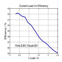
Fig 2 Efficiency Vs Heavy Load
