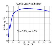
Fig 1 Efficiency Vs Light Load
