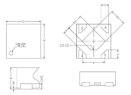
COMMON DIMENSIONS (UNITS OF MEASURE=MILLIMETER)
